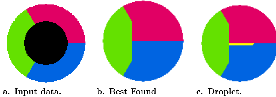
Figure 3.11: Triple-junction inpainting benchmark [117, 119]. Panel (a) shows the input: pixel labels are fixed on a circular boundary, while the interior (black region) is unknown. Panel (b) shows a lowest-energy configuration found by SpinGlassPEPS.jl . Due to the grid-based discretization, the energy function is mildly anisotropic, which can bias reconstructed interfaces toward axis-parallel directions [117]. Panel (c) highlights a droplet, i.e. , a localized set of Potts variables that can be collectively relabeled to produce an alternative low-energy solution. Such droplets provide a compact description of near-degeneracies and are useful for characterizing solution diversity in subsequent benchmarking.
