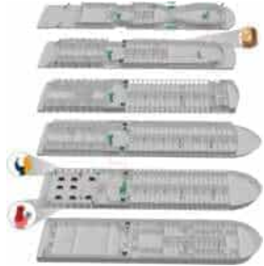
FIGURE 12. Experimental layout on a real-word passenger ship. Sensors are deployed at the locations colored red and green. We select the sensors at the green-colored locations as the landmarks.
