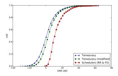
Fig. 2. Comparison of the SINR empirical cumulative distribution function for all UEs
